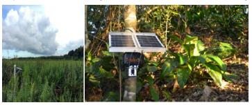
Fig. 1: ARBIMON biodiversity monitoring stations will be the core of a global network. The solar powered stations include an ARBIMON recording device (Android smartphone) with a cellular data plan, which is used to upload recordings in real-time to the ARBIMON II bioacoustics analysis platform. In addition, a companion app uploads status reports on the state of the battery, cellular connectivity and recording collection and upload. Photo: Sieve Analytics.
