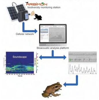
Fig. 2: Data acquisition, transfer, storage and analysis from the ARBIMON biodiversity monitoring station to the ARBIMON II bioacoustics analysis platform.
